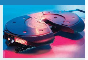
concern that, since they are under the rear axle and out of the way, it's a case of 'out of sight, out of mind'. VBG recommends visually inspecting coupling equipment at least weekly, and more frequently where vehicles have been overloaded, looking for cracks, corrosion and deformation. If damage is evident, then – since welding and straightening are not allowed – parts must be replaced.
